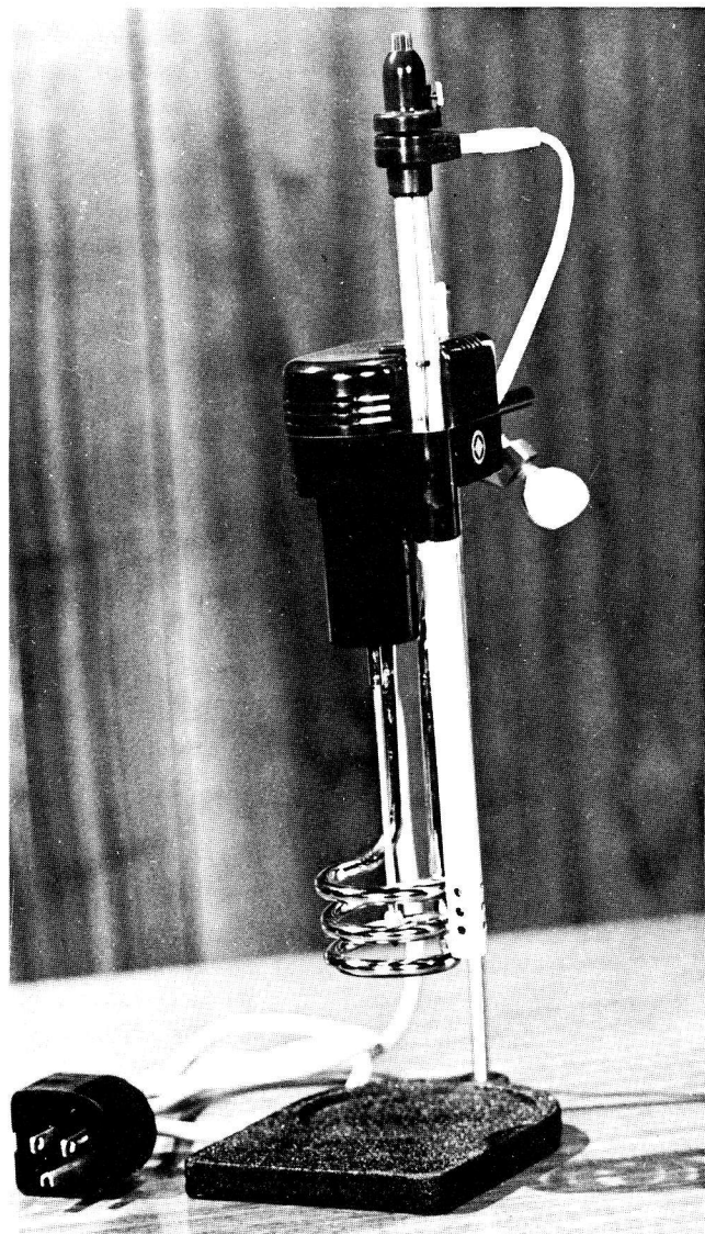
FIGURE 3 Bronwill Model 22 Constant Temperature Circulator, Jr.
