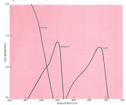
Sensitivity=reciprocal of exposure (ergs/cm²) required to produce a gross density of 1.0 above fog.
