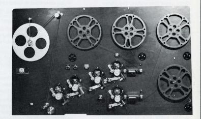
HFC slitters are engineered to produce proper slit width from processed positive motion picture film. The HFC sprockets are full fitting, and as such are calculated to accommodate the normal percentage of stretch found in positive film immediately after processing.
