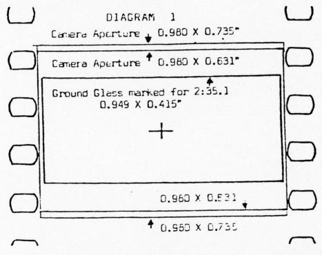
From the flat full frame negative an optical squeeze to 2.35:1 is applied in printing. Thus Squeezed Prints, Interpositives and Interdupes can be made from the flat negative.
